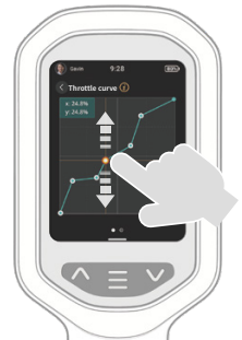
In Custom mode, hold down the trigger and tap a coordinate point, then drag your finger up or down to adjust it.
